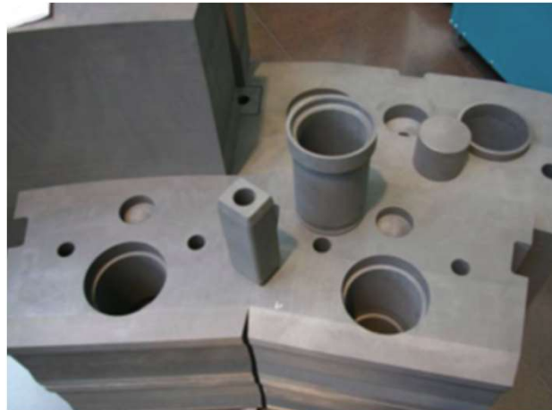
Fig. 2: Nuclear Graphite Components
