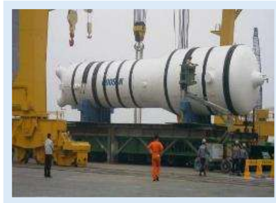
◆ Kori #1 Steam Generators
