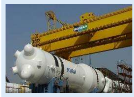
Sequoyah #1,2 Steam Generators
