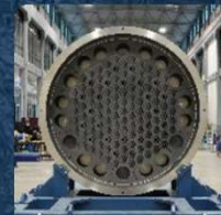
Full-Diameter Manufacturing Demonstration Unit, 32,000 lbs, 3.2 m Diameter
