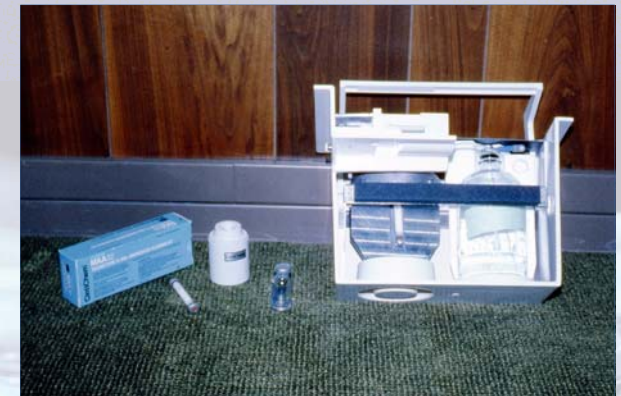
Mo-99 Generator Cutaway with Kit, Vial, and Shield
